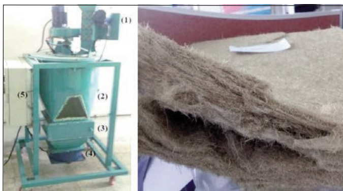
Fig. 2. Airlaid machine and Kenaf panel K1
